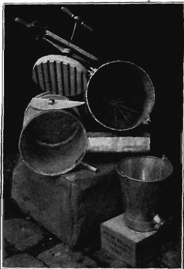
Fig. 7.—Metal Wax-press showing parts.
