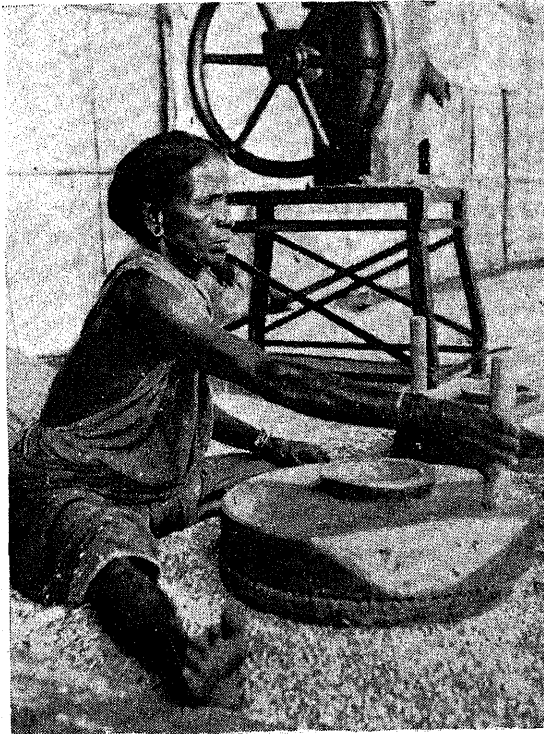
A flat wooden chakti used for husking paddy. Turns out unpolished rice. Can husk 4 maunds a day of 8 hours. Is worked by one woman. Cost Rs. 12-8-0.
