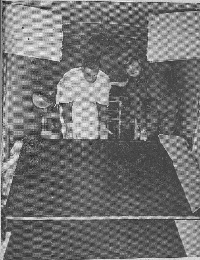
Getting the theatre ready. The theatre itself is in a lorry, behind which is a trailer containing all the necessary equipment. Here are two officers, one a surgeon, placing in position the floor connecting the lorry with the trailer.
