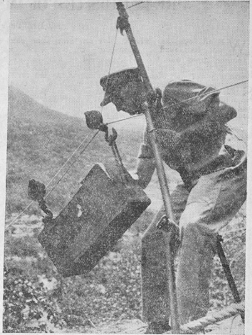
JUNGLE WARFARE TRAINING SOMEWHERE IN INDIA.—Officer unloading ammunition from the hoist improvised from a Bren-gun tripod.
