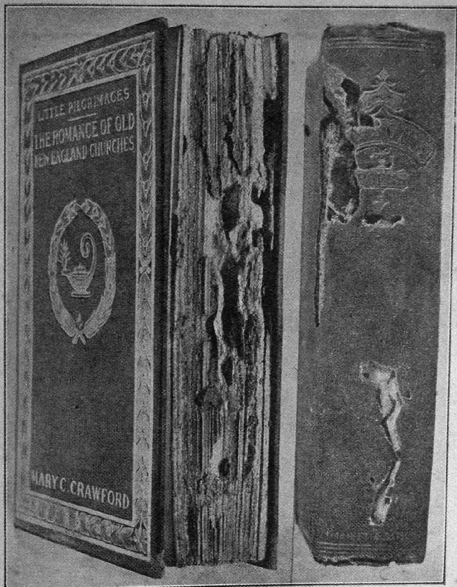
TWO BOOKS SHOWING EXTERIOR EVIDENCE OF ATTACK BY SUBTERRANEAN TERMITES.
