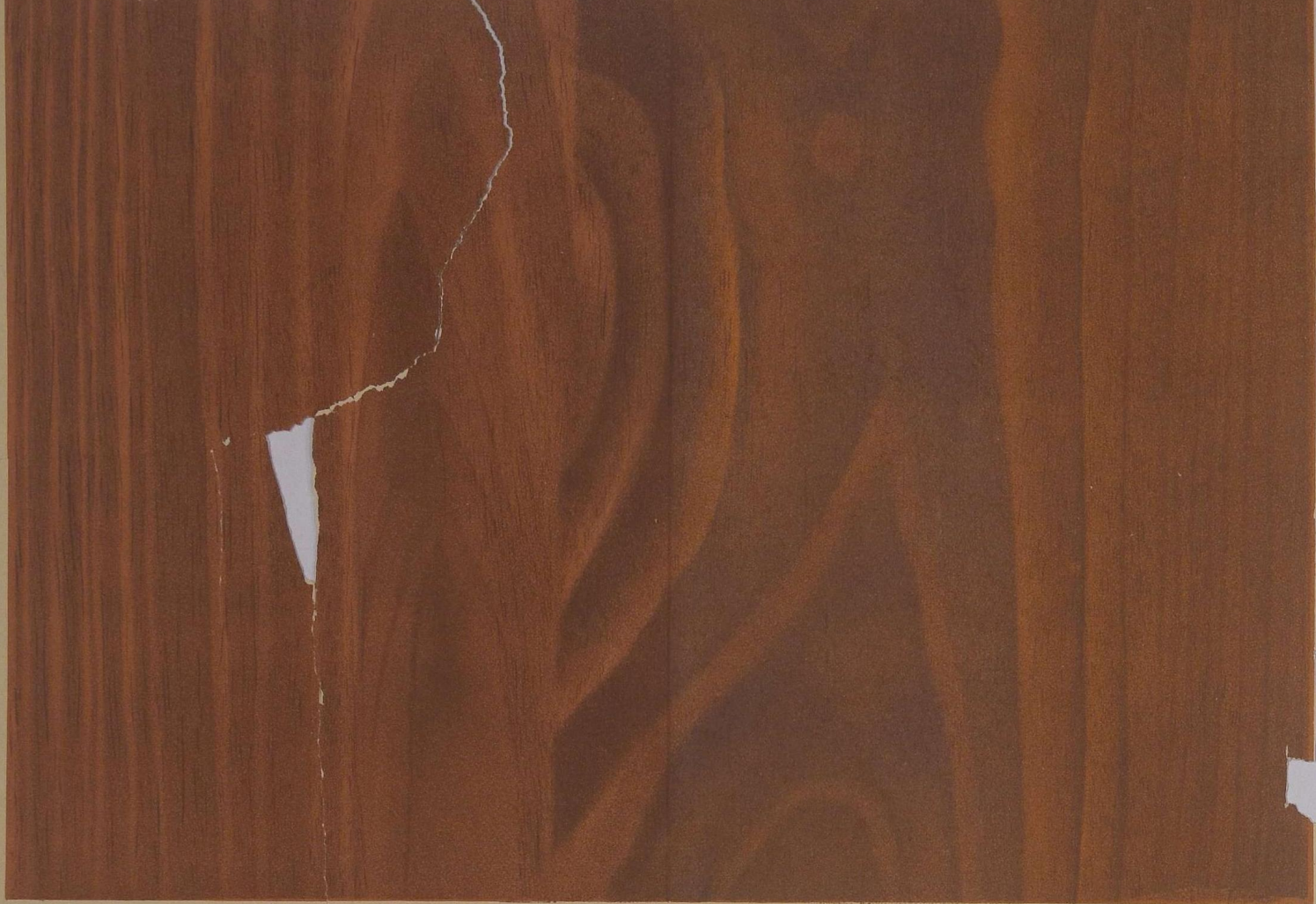
41.— Bischofia javanica . (Red Cedar.) A deciduous tree found in Kumaun and Burma. Weight 47\frac{1}{2} lbs. per c. ft. Wood rough, and moderately hard. In Assam it is highly esteemed and used for bridges &c. MANSON.
