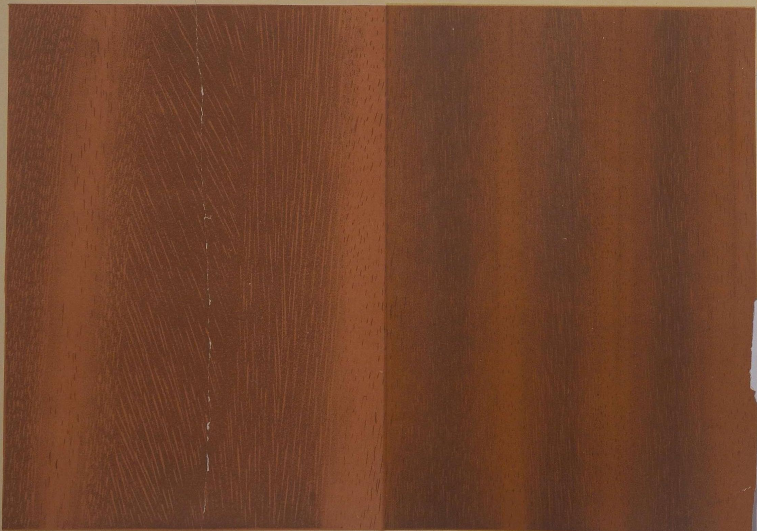
42.— Artocarpus ... A lofty deciduous tree, met with in Eastern Bengal, Burma, and the Andaman ... to brown, moderately hard, even-grained, rough, durable, and ...
