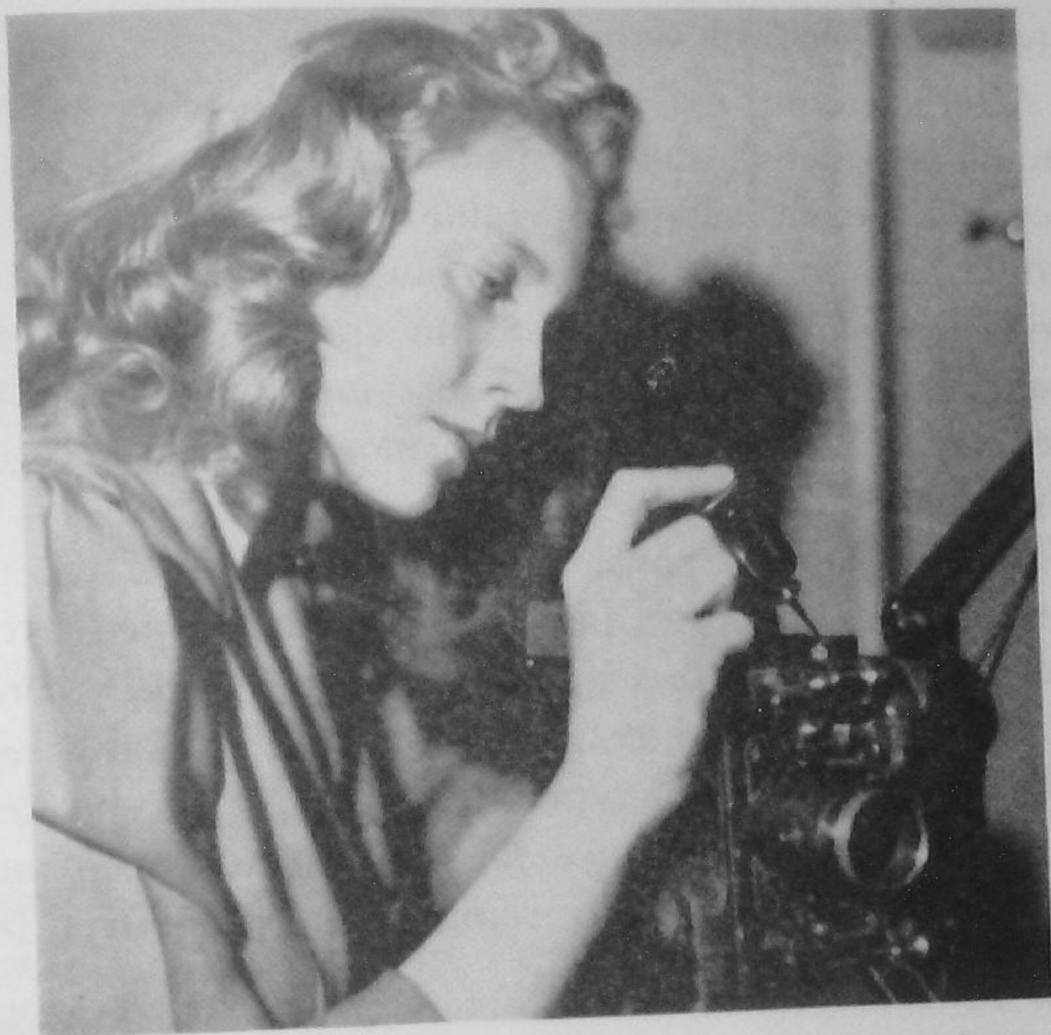
Fig. 13. Regular lubrication is important for long life of the projector.
