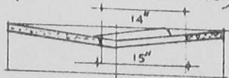
DETAIL PLAN OF SQUATTING SLAB (BORE HOLE LATRINE) ② & ③
