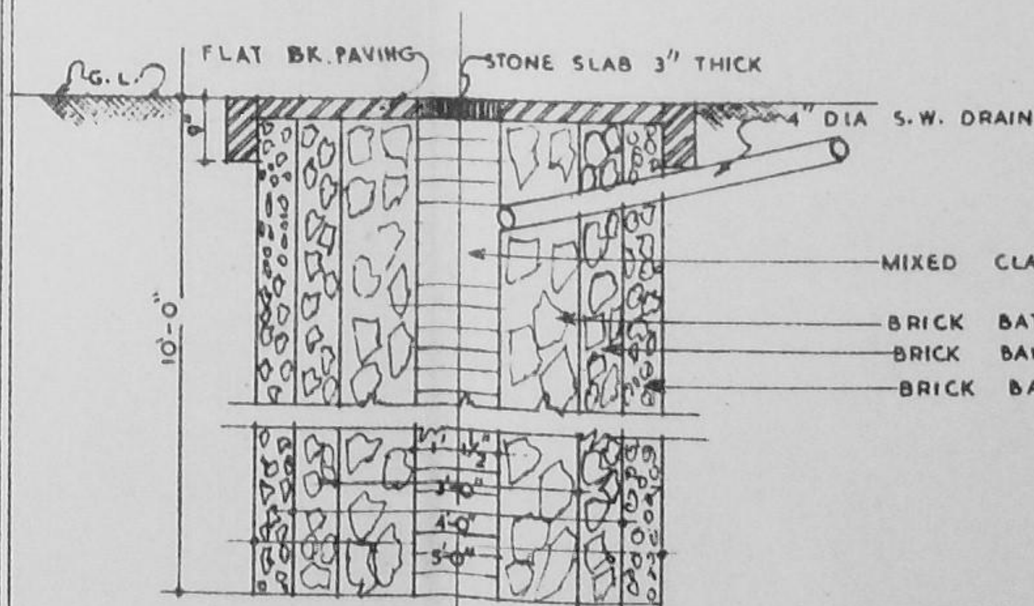
1/2" DETAIL OF SOAKAGE PIT 5' DIA: 10' DEEP
