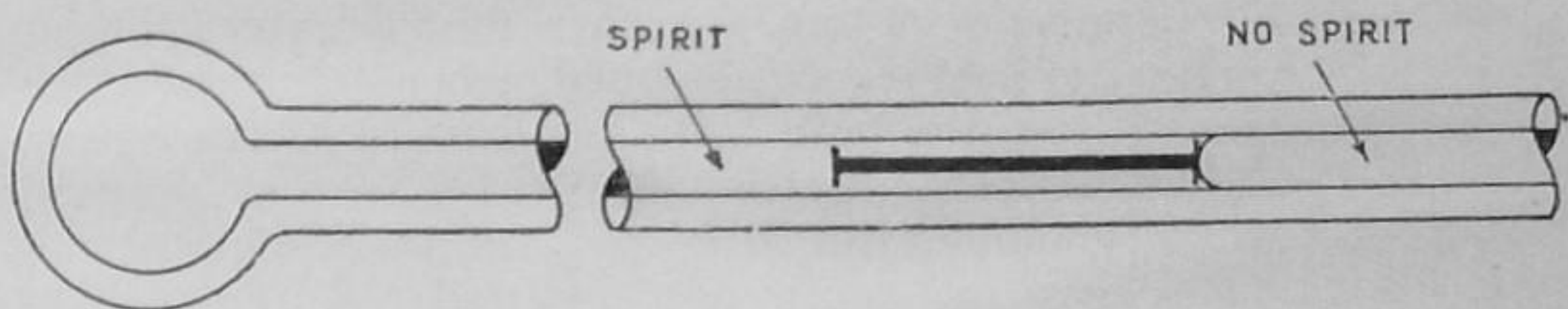
FIG. 11.—MINIMUM THERMOMETER CORRECTLY SET.
