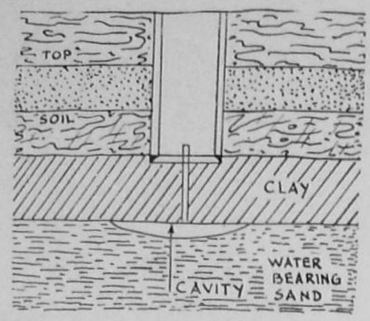
held up between the intervening layers. Hence, there may be a third or even a fourth layer. The water contained in the lower strata of the sand will obviously be under pressure and would rise if we drill a hole through the intervening clay. The water thus held up is known as the "confined water," from which cavity wells draw their supplies.
