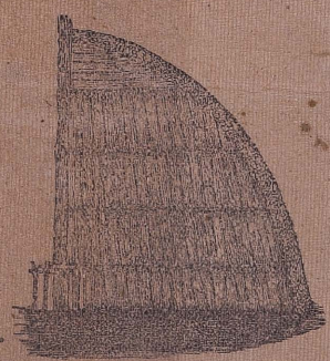
Section of one-half of the Kiln.
