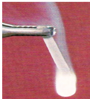
Iron wool (made into thin fibres) burns in oxygen to produce both heat and light energy.
