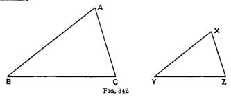
Thus, if  $\angle A = \angle X$ ,  $\angle B = \angle Y$ , and  $\angle C = \angle Z$ ,  $\triangle ABC \parallel \mid \triangle XYZ$ .
