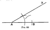
Proceeding as before, the arc which has centre B and radius 1.5 cm. does not cut the straight line AX.
