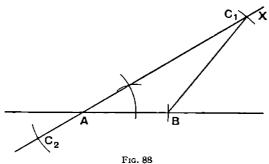
Proceeding as before, the arc which has centre B and radius 5.9 cm. will be found to cut AX (at  $C_1$ , say) and XA produced (at  $C_2$ , say).
