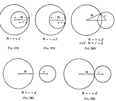
To construct a direct common tangent to two circles.
