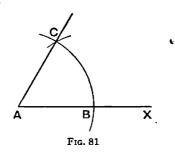
Suppose it is required to construct, at the point A, an angle of 60° with the straight line AX.
