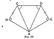
In the right-angled  $\triangle s$  ABC, AED,  $\angle ABC$  and  $\angle AED$  are the right angles (given), BC=ED (given),  $AC=AD ( : \angle ADC = \angle ACD )$ :  $\therefore$   $\triangle s \stackrel{ABC}{AED}$  are congruent (RHS). ∴ AB=AE.
