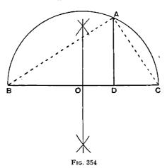
**Construction.** Along a straight line, mark off BD, DC equal to the given lengths.
