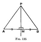
Given two points A and B, M the mid-point of AB, and P any point on the perpendicular bisector PM of AB.
