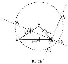
In the figure the two loci are shown by dotted lines. It will be seen that there are four possible positions for P, namely  $P_1$ ,  $P_2$ ,  $P_3$ ,  $P_4$ .
