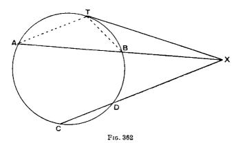
Given two chords of a circle, AB, CD, produced to meet at X, and a tangent XT touching the circle at T.
