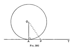
Given a circle, centre O, a point A on the circle, and the straight line AT perpendicular to OA.
