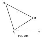
On a given straight line to construct a segment of a circle to contain a given angle.
