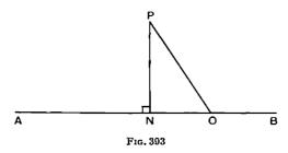
Given a straight line AB and a point P outside it; N is the foot of the perpendicular from P to AB; P is joined to any other point O in AB.
