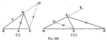
Given a triangle ABC, and a straight line through A which divides BC, internally in Fig. 332 (i), externally in Fig. 332 (ii), so that BX: XC=BA: AC.
