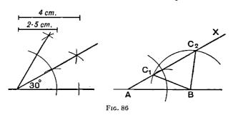
First draw the data on the left. (The given angle of 30° may be drawn either by means of a protractor or by a geometrical construction.)
