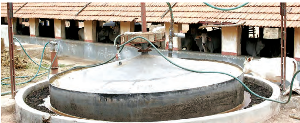
Fig.11.11-Biogas (Gobar gas) plant
