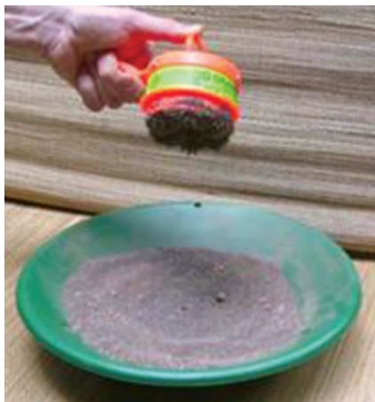
Fig. 10.3. Separation of Iron filings from sand using magnet
