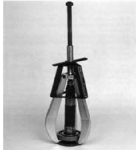
Fig.15.1 - Bearing removal using puller
