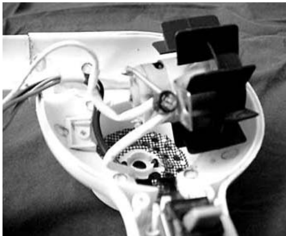
Fig.13.9 - Hair dryer motor
