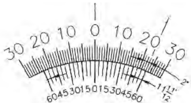
Fig 3.20 Reading with vernier bevel protractor
