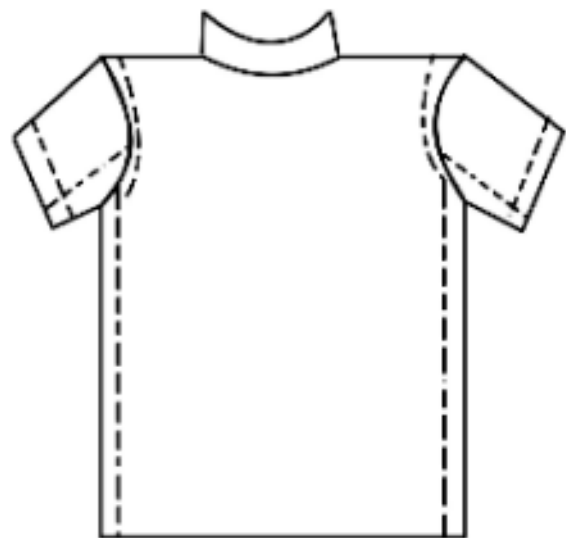
Finishing side seams
