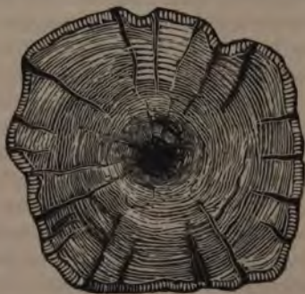
Fig. 4. Showing Radial and Concentric Splits.
