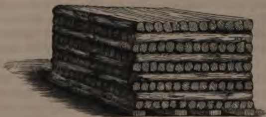
Fig. 5. Pile of Wood raised on Bricks.
