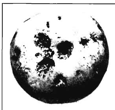
FIG. 15.- Severe injury caused by T. dimidiatus to the cap of a large button. Nat. size.
