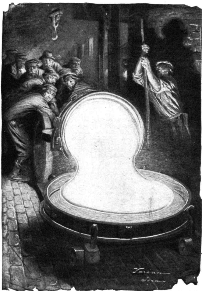
CASTING A GREAT LENS AT JENA. THE CRITICAL POINT
