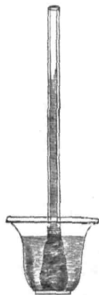
FIG. 50.—APPARATUS* TO SHOW THE PRO- CESS OF OSMOSIS.
