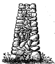
A SECTION OF WALL IMPROPERLY LAID.
