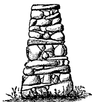
A SECTION OF WALL WELL LAID.
