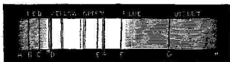
FIG. 2.—Diagram of the solar spectrum, showing the order of colour and the position of the principal absorption lines.
