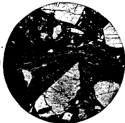
FIG. 235.—Eutaxite. Microscopic Fluidal Structure in Pitchstone. Kastelruth, South Tyrole.
