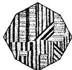
FIG. 154.—Twinning Lamination in Leucite.
