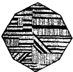
FIG. 232.—Twinning Lamination in Leucite.
