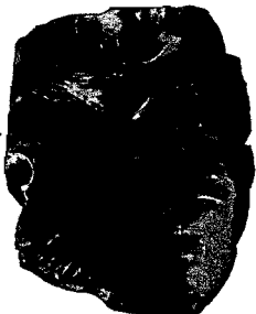
FIG. 233.—Conchoidal Fracture (1/2 Natural Size). Obsidian, Iceland.
