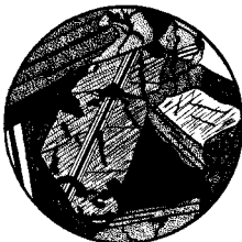
FIG. 102.—Simple Twinning Lamellae in Augite.
