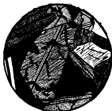
FIG. 300.—Simple Twinning Lamellæ in Augite.
