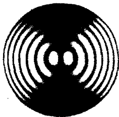
FIG. 129.—Interference Figure of a Biaxial Crystal Perpendicular to an Optic Axis.
