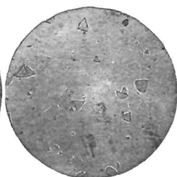
FIG. 45.—Lower Index of Crystal in Canada Balsam with Raised Tube.
