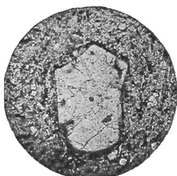
FIG. 50.—Mineral with Low Index in Canada Balsam.
