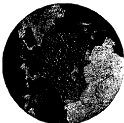
FIG. 352.— Perthitic Intergrowth of Orthoclase and Plagioclase.
