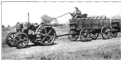
FIG. 164.—Tractor with remote control used for hauling wagons.
