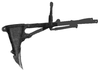
FIG. 82.—116" furrow-opener, with opening trip release.
