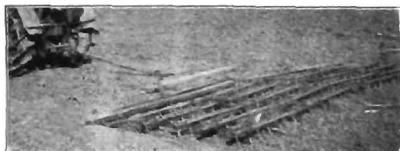
FIG. 49.—Three-section, flexible, peg-tooth harrow.
