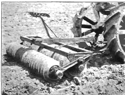
FIG. 73.—A ridged roller soil pulverizer hitched direct to tractor draw-bar.
