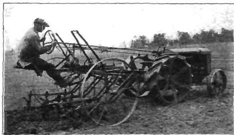
FIG. 293.—Cultivator attachment with remote control for early cultivating.
