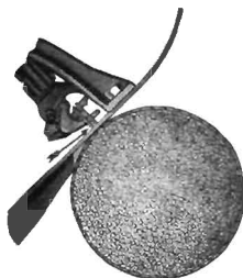
FIG. 122.—Knotting device drawing twine around bundle.
