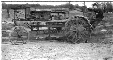
FIG. 169.—Road-drag, suspended under a motor cultivator.
