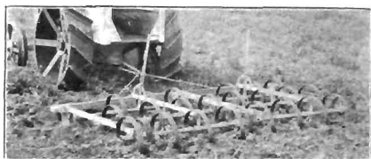
FIG. 54.—A spring-tooth harrow with proper tractor hitch.
