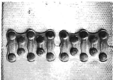
FIG. 305.—Metal belt fastener securing both ends of belt.
