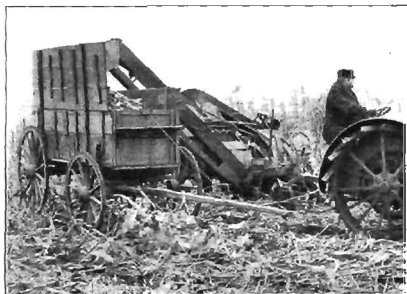
FIG. 172.—Corn picker, with ear-wagon being drawn by single tractor.
