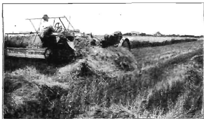
FIG. 117.—Tractor binder in one unit combination with operator of both machines on the seat of the binder itself.
