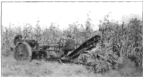
FIG. 137.—Corn binder and tractor, with one operator for both.
