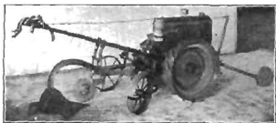
FIG. 294.—Garden tractor with plowing attachment.
