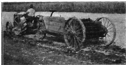
FIG. 159.—Spreader, with beater on rear axle.
