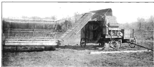
FIG. 151.—A special thresher used in combination with a header, making a combined harvester and thresher unit.
