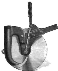
FIG. 79.—Concave side of closed-delivery disc furrow-opener.
