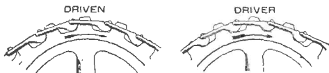
FIG. 316.—Detachablc sprocket chain should be run as shown. Hooks up and running first.
