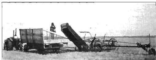
FIG. 142.—Header in use with header large, both being drawn by tractor.
