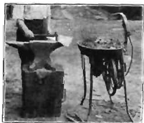
FIG. 39.—Hammering soft-center steel share for sharpening.
