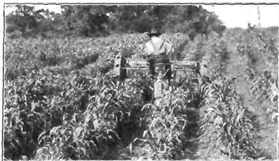
FIG. 280.—Engine cultivator (pivot axle type).
