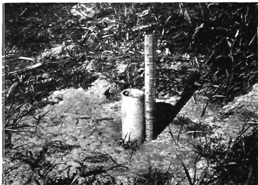
FIG. 96.—Pipe heaved nearly 6 inches during winter of 1915-1916.
