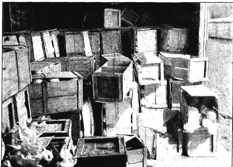
FIG. 185. Condition of improperly loaded and braced car on arrival in market
