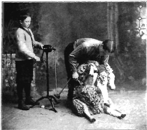
FIG. 141.—SHEARING SHEEP BY MACHINERY, SHOWING POSITION OF THE SHEEP, SHEARER, AND THE MACHINE.
