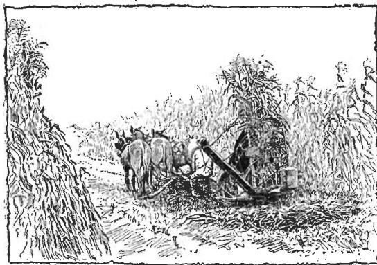
FIG. 68.—Cutting corn with a harvester that has an attachment to carry the stalks until a bundle is formed.
