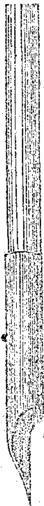
Fig. 75. Cutting Tool, for finishing between the teeth of Vulcanite cases.
