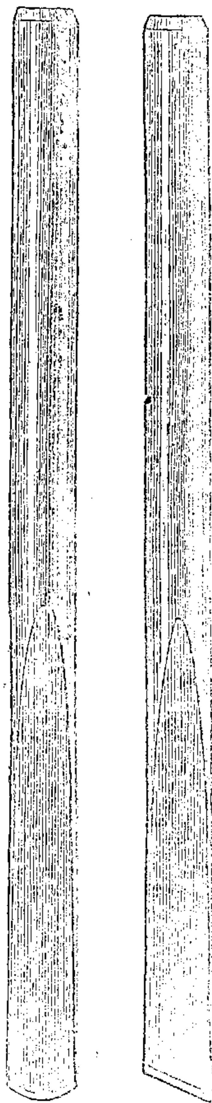
Fig. 19. Punches for dressing Zinc Models.
