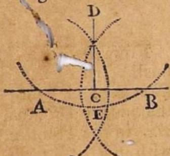
4. Upon the End B of a given right Line BA, to raise a Perpendicular.
