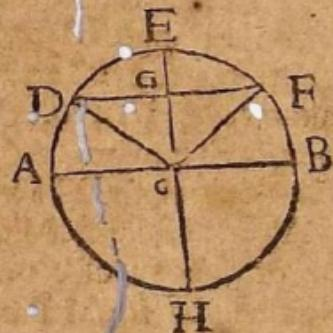
Root of which, *viz.* .8 is equal to DG, and this doubled gives 1.6 equal to DF, which multiply'd into .3, the half CG produces .48 for the Area of the Triangle DCF. Then, from .92727789 for the Area of the Sector DCFE taking .48 the Area of the Triangle DCF, there will remain .44727789 for the Area of the Segment DEF D, and this taken from 3.1416, the Area of the whole Circle, there will remain 2.69432211 for the Area of the other Segment DHFD, whose versed Sine is 1.6.
