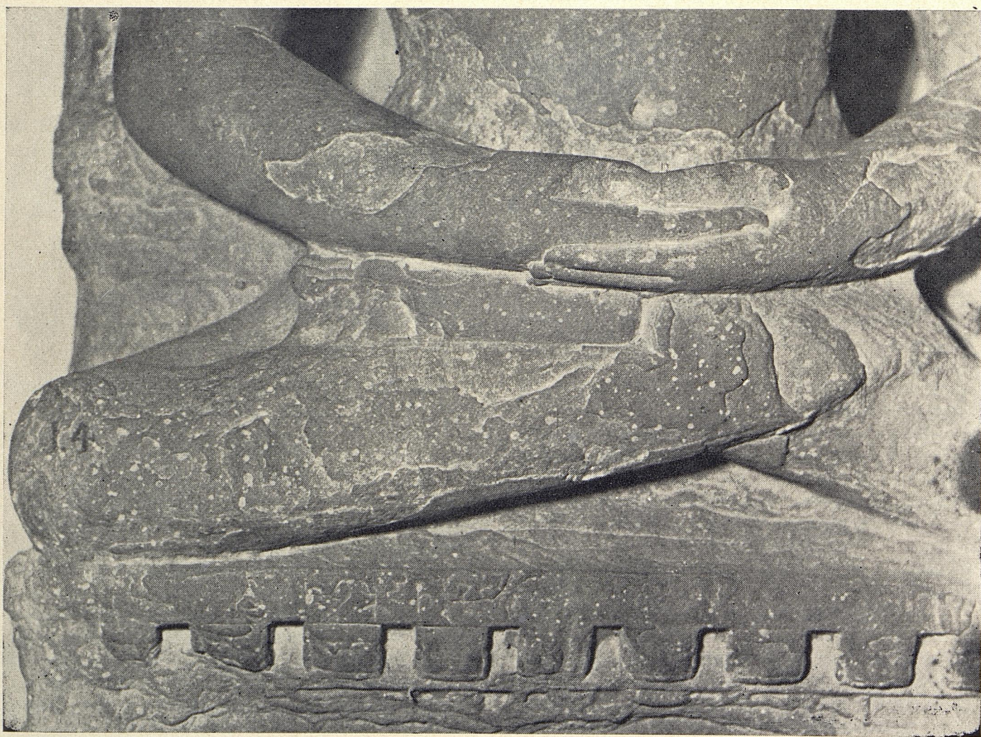
Figure 7. Because of the action of salts contained inside stone, the stone surface is damaged and becomes powdery.
