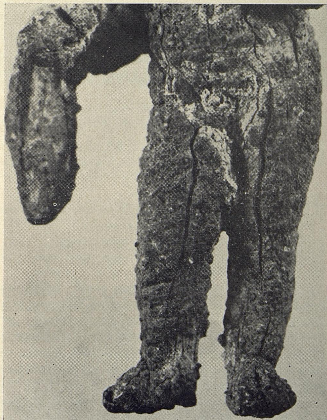
Figure 4. Copper objects when excavated are covered with copper corrosion products like carbonates, chlorides, oxides and sulphates of copper.
