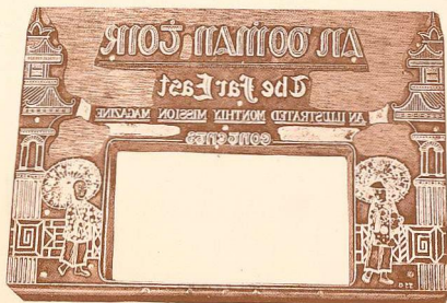
Fig. 27—A finished line-block, opening pierced for type.
