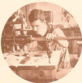
Fig. 24—Router, a quickly-revolving tool for cutting away the waste portions on a block.
