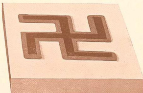
Fig. 18—Model of Zinc Plate after first powdering to protect sides of lines.
