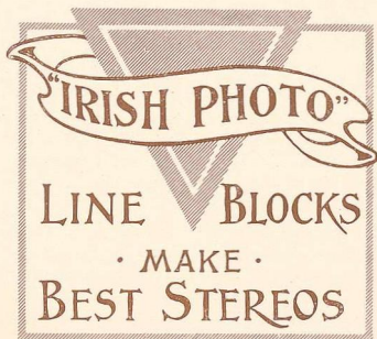
Fig. 62—Combined line and “half-line” (65 lines to inch) on one piece of zinc.
