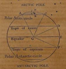
Let w be the unknown arch of the Meridian compreheaded above the arctic polar circle A B C, and let D E F be the arch of the same Meridian comprehended between
