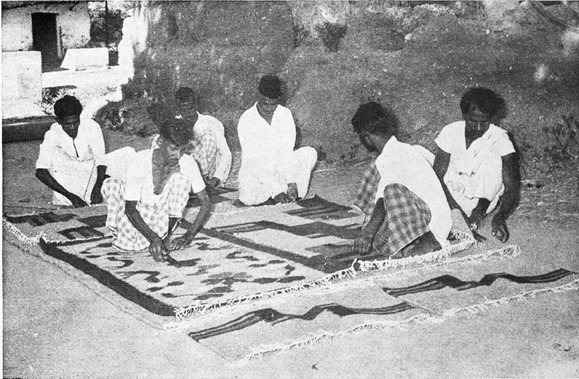
After removing the drugget from the loom it is spread on the ground to bind the fringes hanging on two opposite sides. The background is a house of a weaver in very bad condition which reflects the social and economic condition of the Walajapet weavers.
