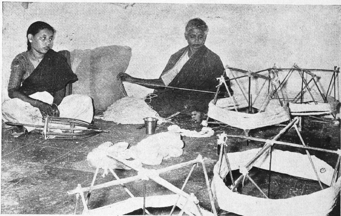
In the house of the woman twister, the cotton yarn of 10 counts for 8 plys is spread into four branches on the two drawing wheels. Note the woman twister holding cotton yarn by her left fingers and drawing the thread by her right.
