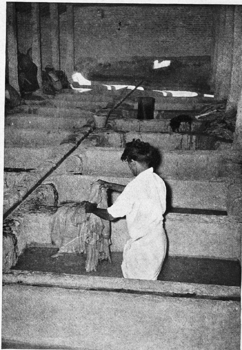
The cheap quality wool viz the lime wool is soaked in the tannery at Vaniyambadi. Note the worker removing the cheap quality hide from the lime pit.
