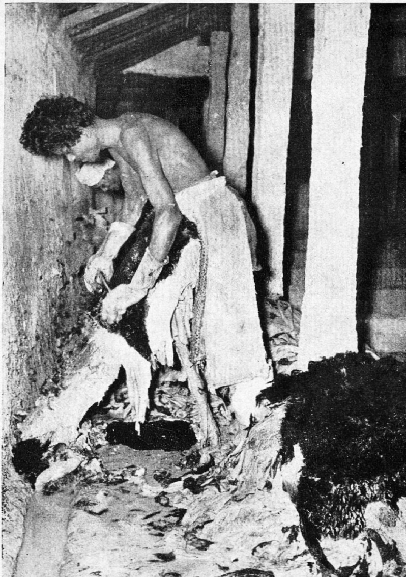
Placing the lime soaked skin on a vertical wooden plank, the worker wearing gloves to protect his hands from lime is busy removing the wool from the hide with a peculiar type of knife.
