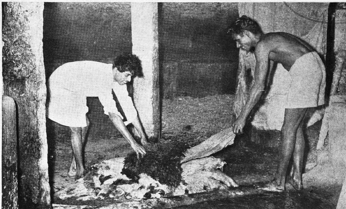
The person at the right is holding a piece of cloth, in a tannery at Vaniyambadi, where there is paste prepared of sodium sulphate in a pit which is seen partially at the right corner and the person at the left is pasting the fleshy side of the hide.
