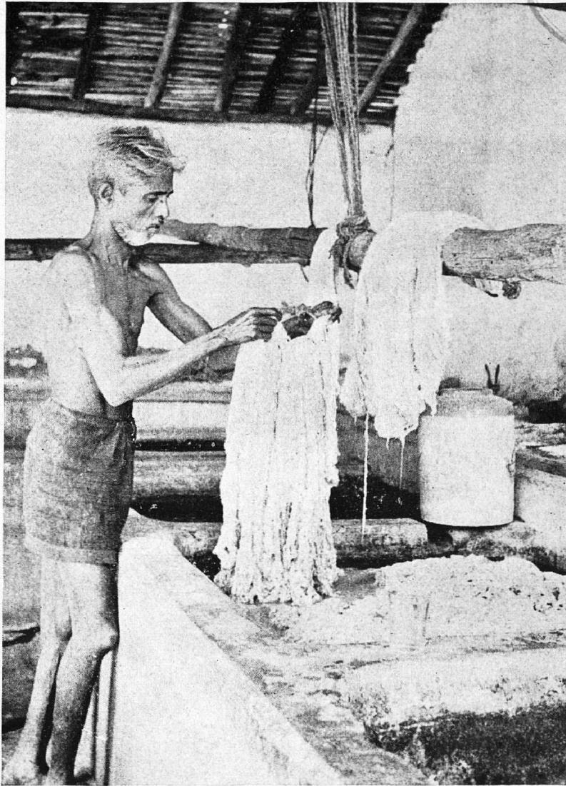
In the Drugget Factory at Walajapet, the dyer picks up the hanks from the tub, washed in the soap solution. (Note the China clay pot and glass used for mixing the chemicals)
