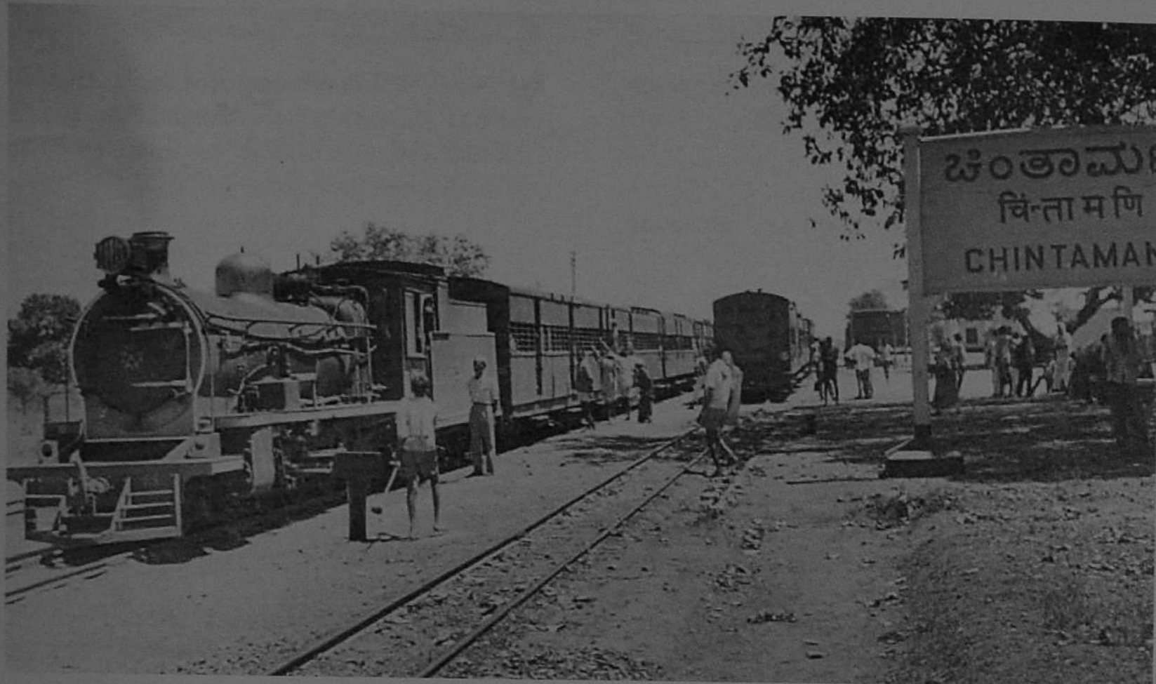
Southern Railway ES 505, a 4-6-2, design built by M/s Kerr Stuart & Co. Ltd., Stoke-on-Trent, in 1922. This locomotive was rebuilt with super heater.
