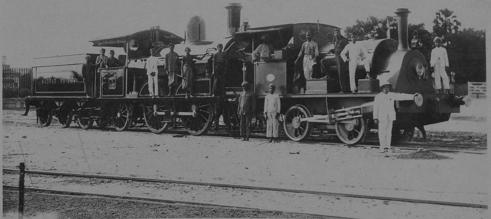
Two locomotives of Madras Railway A 0-4-2 'H' class locomotive No. 245, built by M/s Kitson & Co., Leeds in 1877, being pulled by a shunting locomotive No. 1 of 'PW/E' 0-4-0 ST class, built by M/s Hudswell Clarke & Co., Leeds in 1905.
