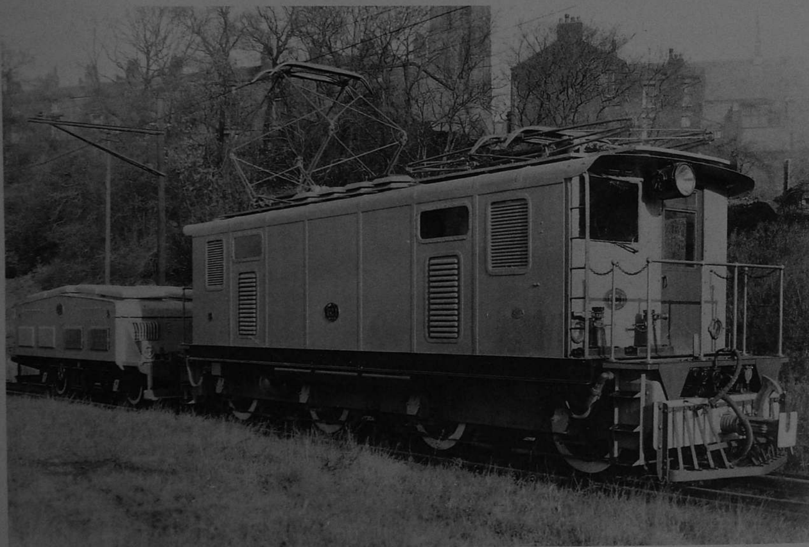
EG 1 (later YCG 21900), B+B design Metre Gauge Electric Locomotive of South Indian Railway along with battery tender ET 1. These were built by M/s R & W Hawthorn, Leslie & Co. Ltd., Newcastle-upon-Tyne and M/s The English Electric Company, Preston & Rugby respectively in 1930.
