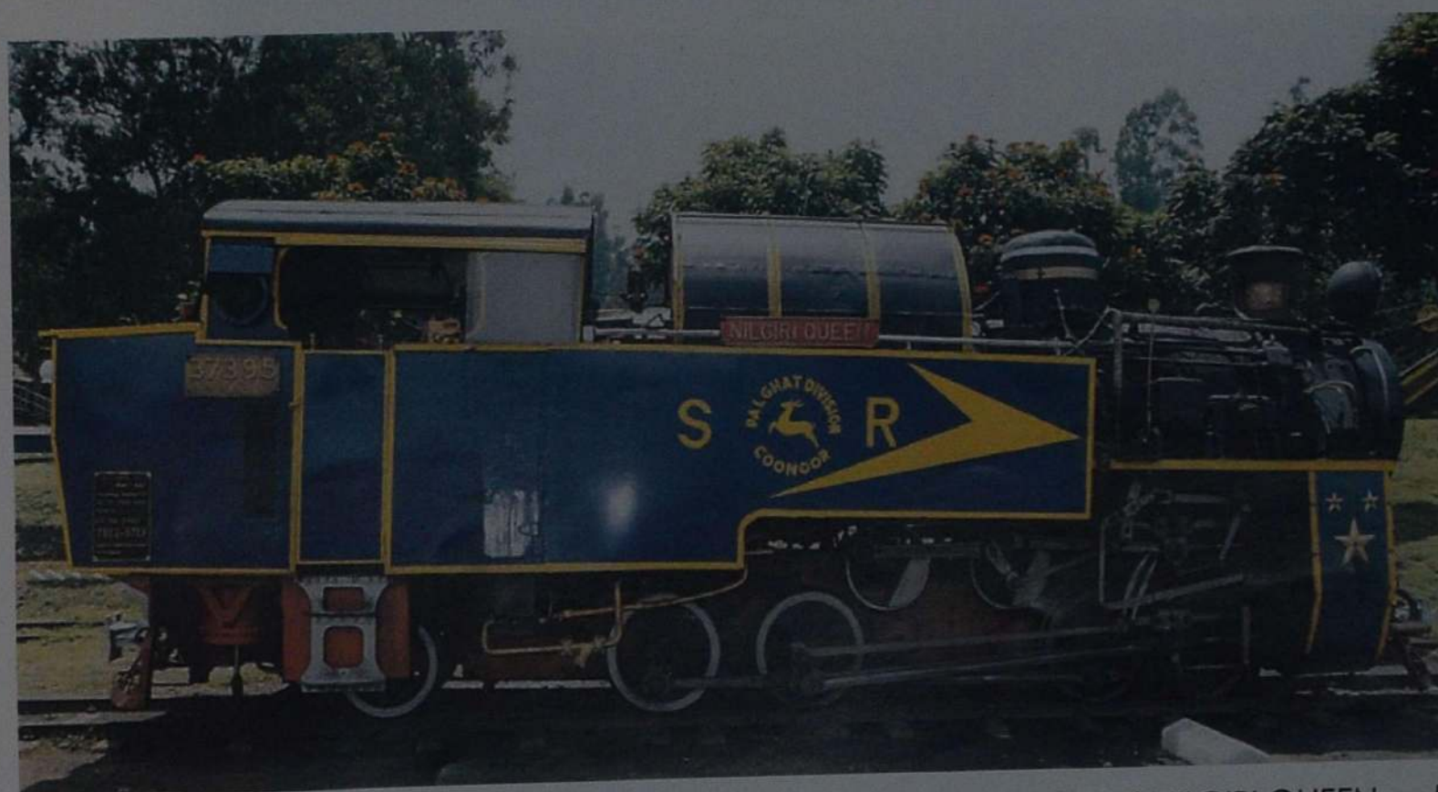
X-37395 after its retrofitment with oil firing system in 2003. It has been named NILGIRI QUEEN and works from Mettupalayam to Coonoor.
