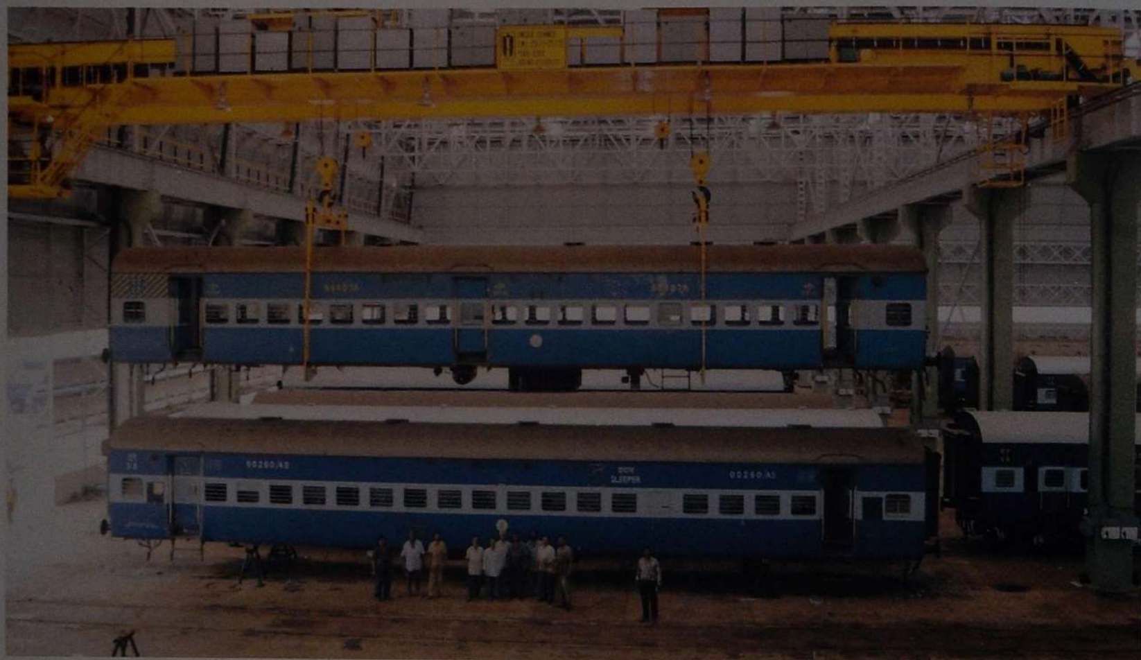
New Carriage Repair Shops at Perambur. Note the height of the overhead crane enabling it to lift one coach above the other thereby improving flexibility.
