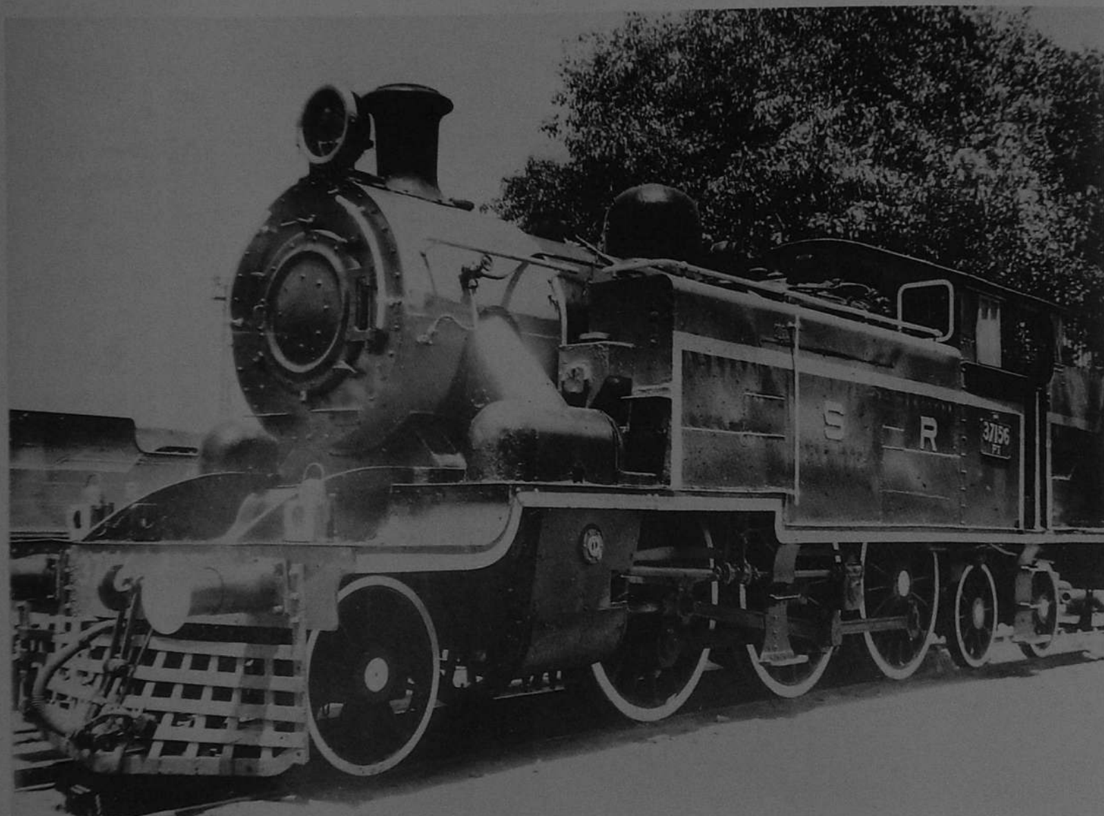
PT 37156 (earlier PT 11 of SIR) in Southern Railway livery. This locomotive of 2-6-4T design was built by M/s Robert Stephenson & Co. Ltd., New Castle & Darlington in 1936.
