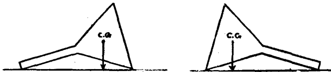
Fig. 43. Neutral Equilibrium C. G - Centre of Gravity
